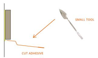
Then using the flat end of the small tool, scrape 'forwards', cleaning off any remaining adhesive (refer to the diagram below for scraping 'forwards'). This is important because scraping in the wrong direction presses the adhesive into the wall. The correct method will leave the remaining adhesive 'lifted', allowing for easier cleaning.
