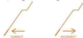
Using water and the 50mm brush (or sponge) clean away all remaining adhesive. Do not leave a groove between the moulding and the wall, as this will show up when painted. A flush corner with no surface adhesive is the ideal result, for the best finish.
